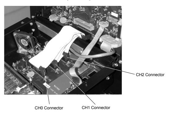
**Figure 4-10 Channel Connections**
